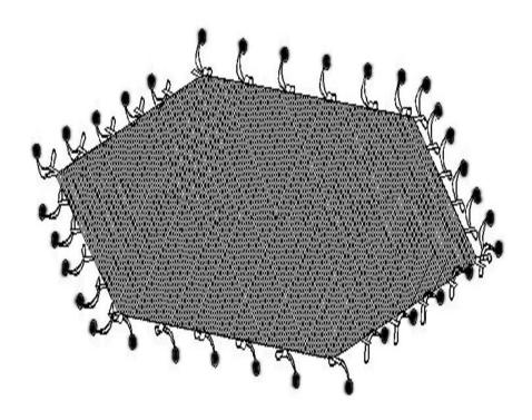
Step 4:fasten the bungee cords to the frame tube, first fasten the two bungee cords on every corner as following figure, then fasten the remaining cords in an alternating manner on opposite sides of the trampoline to ensure even tension
