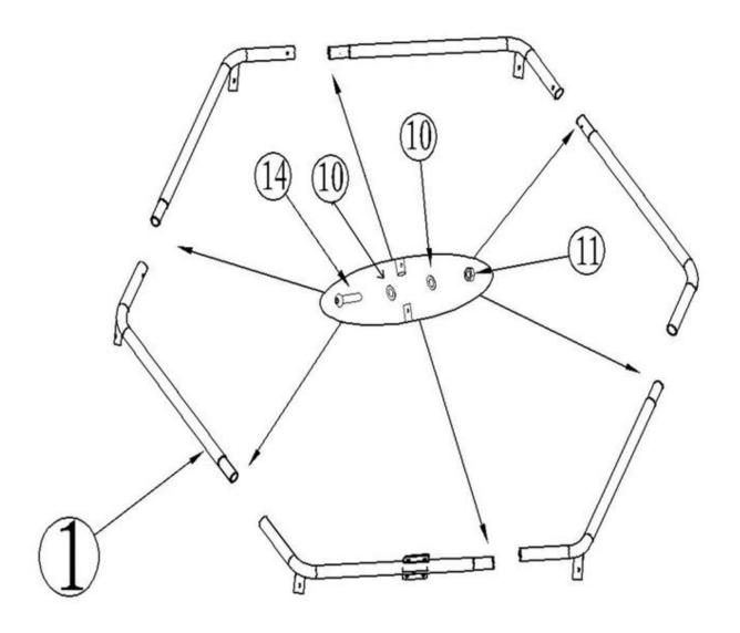
Step 2:Remove the black caps that cover the leg holes. Assemble legs to frame tubes by screws according to following picture.
